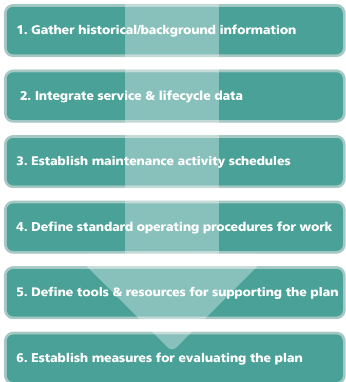
Figure 4.2 – Steps in developing a Maintenance Plan
